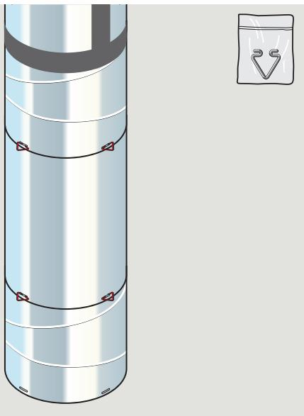
**ENGLISH:** Connect tunnel assembly with the clips supplied.
