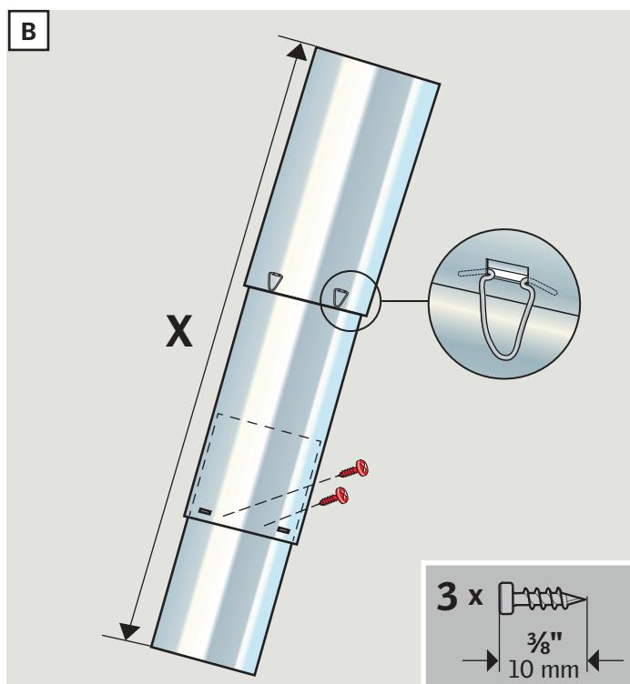
**ENGLISH:** With more tunnel sections, assemble the upper sections with the tunnel clips provided and reduce the length of the tunnel assembly by increasing overlap at the bottom. Secure the joint with three of the 3/8" (10 mm) screws (B). Length of tunnel should not exceed 30 ft. (9 m).
