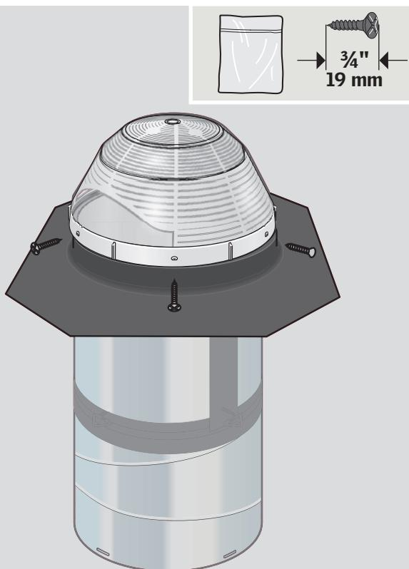
**ENGLISH:** Place sun curve on top of tunnel assembly (size 022 only). Install dome by aligning holes and securing with the  $\frac{3}{4}$ " (19 mm) screws provided. Do not overtighten the screws.
