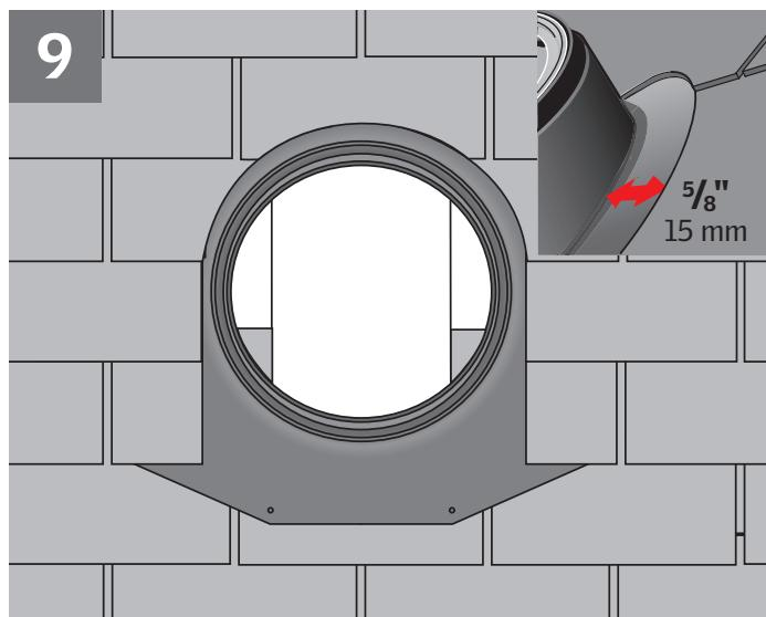
**ENGLISH:** Reinstall roofing material over the flange. Leave a  $\frac{5}{8}$ " (15 mm) channel for water to run off.
