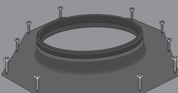
**ENGLISH:** Install and secure the flashing with 1" (25 mm) screws provided.
