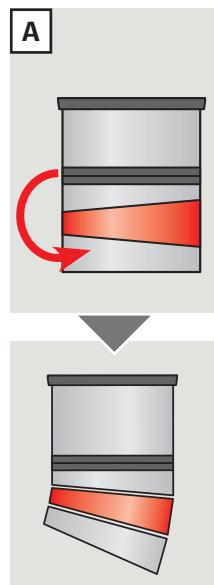
**ENGLISH:** Adjust the angle of both elbows so that they point directly against each other **(A)**, **(B)**. Elbows can be damaged if excess force is applied.
