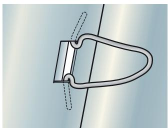
**ENGLISH:** Assemble the rigid tunnel section with tunnel clips provided.
