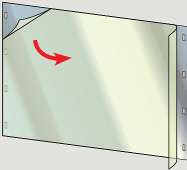
**ENGLISH:** Remove protective film from the 16" (405 mm) rigid tunnel section.
