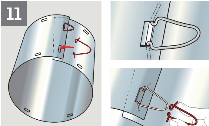
**ENGLISH:** Assemble the 16" (405 mm) rigid tunnel section with tunnel clips provided.
