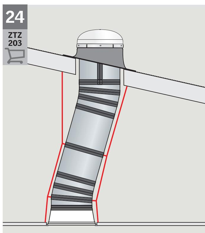
**ENGLISH:** Suspension kit ZTZ 203 may be needed to comply with building codes and safety requirements. If installing the suspension kit, use instructions enclosed with the kit before attaching the diffuser.
