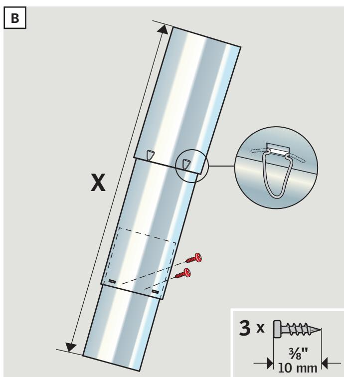
**ENGLISH:** With more tunnel sections, assemble the upper sections with the tunnel clips provided and reduce the length of the tunnel assembly by increasing overlap at the bottom. Secure the joint with three of the  $\frac{3}{8}$ " (10 mm) screws (**B**). Length of tunnel should not exceed 30 ft. (9 m).
