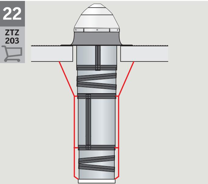
**ENGLISH:** Suspension kit ZTZ 203 may be needed to comply with building codes and safety requirements. If installing the suspension kit, use instructions enclosed with the kit before attaching the diffuser.
