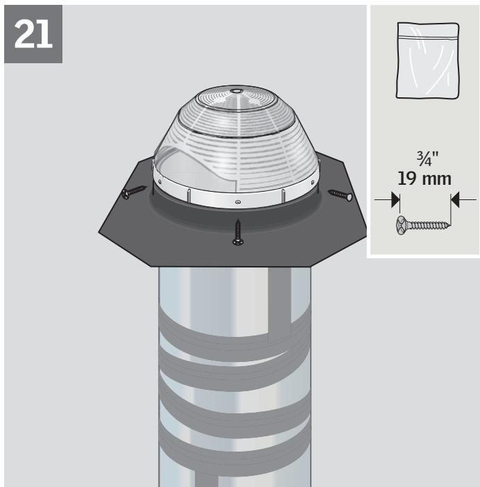
**ENGLISH:** Place sun curve on top of tunnel assembly (size 022 only). Install dome by aligning holes and securing with the  $\frac{3}{4}$ " (19 mm) screws provided. Do not overtighten the screws.
