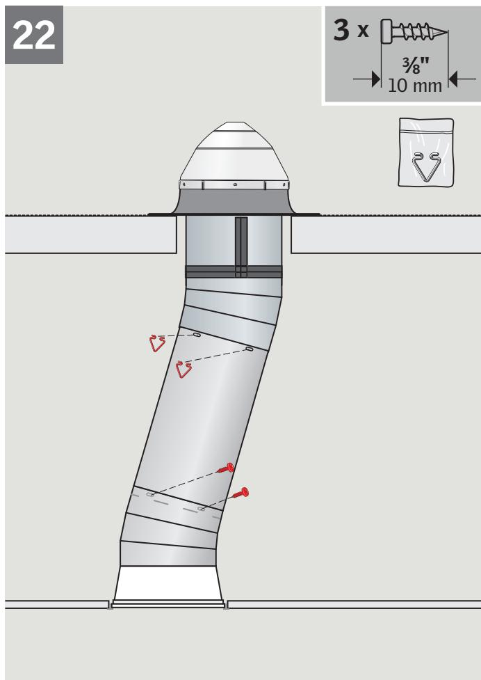
**ENGLISH:** Connect tunnel assembly with the clips supplied. If tunnel section was trimmed or holes do not align, use the screws supplied as necessary.
