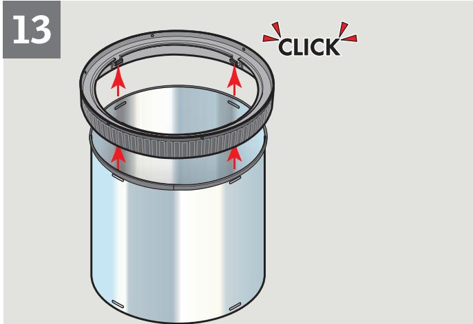
**ENGLISH:** Attach the rigid tunnel section to the pivot ring.
